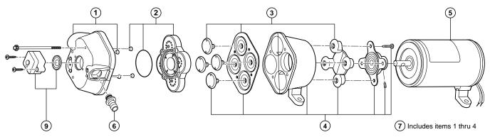
Quite often when a pump is worn or defective the one failed component has overburdened others. To avoid frequent aggravating repairs, Flojet offers service kit assemblies making repairs as quick and easy as possible.
