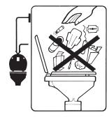
tampons or sanitary napkins. The holding tank and pump should be flushed with several gallons of water after each pumpout. Make sure the battery is fully charged. The dc motor is suitable only for intermittent duty and should not be run for more than 15 minutes continuously. At maximum flow
