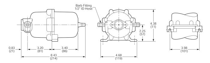
For optimum performance, air pressure may be adjusted to 3 psi (0.2 bar) lower than the pump switch-on pressure.
